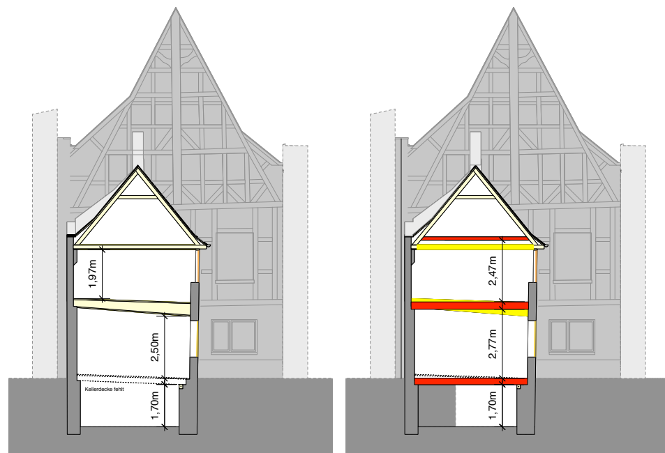
Section Existing Shop / Section investigation / Shop Elevation
