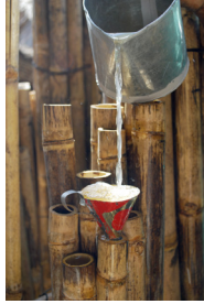
B08 Bamboo set vertically for treatment with Borax solution (Photo: Roswag Architekten)
