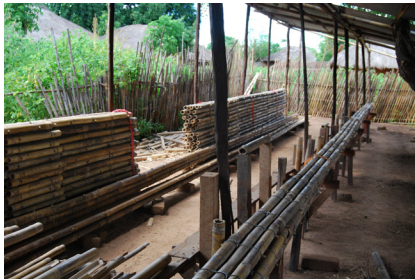
B10 Bamboo workshop: production of triple-layer beams (Photo: Roswag Architekten)
